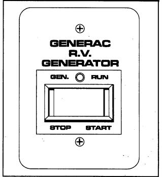
You can also order model 9043, a remote panel which includes the (a start/stop switch, (b) the generator run lamp and (c) and hourmeter. The hourmeter provides a continuous indication of engine-generator operating time. Use the hourmeter for checking off periodic maintenance requirements on the unit.
